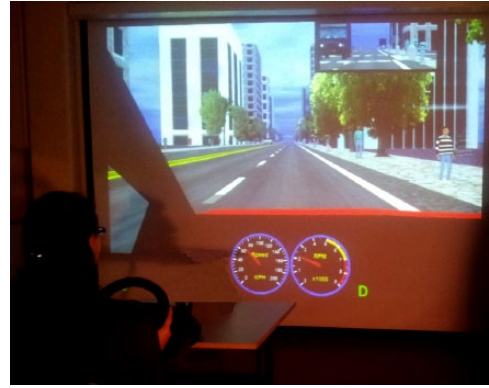
Figure 1. The experimental setup. The participant sat in a clerical chair, holding the wheel, and the scenario was presented on a wide screen in front of her.
